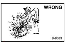
Lead-acid batteries produce flammable and explosive gases.
