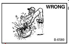
Lead-acid batteries produce flammable and explosive gases.
