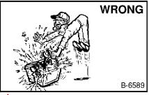
Lead-acid batteries produce flammable and explosive gases.
