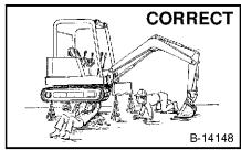
Use the correct procedure to lift and support the excavator. Always lift the blade fully before
