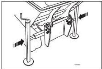
Unscrew bolt A and drive the machine slowly backwards from the quick release system B until support C can be installed.
