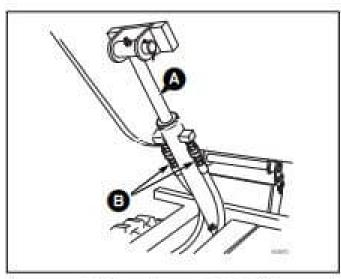
Fit the two supports into the special slots making sure they do not foul the release system.
