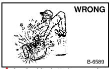
Lead-acid batteries produce flammable and explosive gases.
