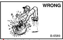
Lead-acid batteries produce flammable and explosive gases.
