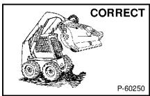
Always install approved lift arm support device when servicing flail cutter. Raise lift arm(s) and tilt Bob-Tach fully forward.
