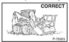
When servicing the forestry cutter always fully lower the lift When arms, place the forestry cutter flat on the ground, engage the parking brake and stop engine.
