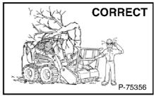
Do Not operate forestry cutter without a Level II FOPS kit installed on the cab of the loader.
