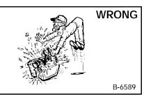
Lead-acid batteries produce flammable and explosive gases. Keep arcs, sparks, flames and lighted tobacco away from lighted
