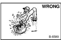
Lead-acid batteries produce flammable and explosive gases.
