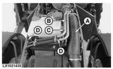
Open the hose clamps, remove air intake line (A) and seal the openings.
