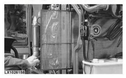
For efficient cooling, the radiator screen must be kept clean.
