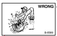
Lead-acid batteries produce flammable and explosive gases.
