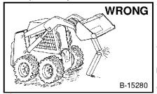
Never work on loader with lift arms up unless lift arms are held by an approved lift arm support dévice. Replace if damaged.
