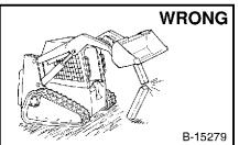
Never work on loader with lift of arms up unless lift arms are held of by an approved lift arm support device. Replace if damaged.
