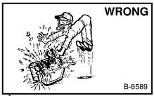
Lead-acid batteries produce flammable and explosive gases.
