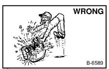
Lead-acid batteries produce flammable and explosive gases.
