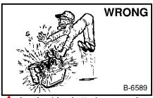
Lead-acid batteries produce flammable and explosive gases.
