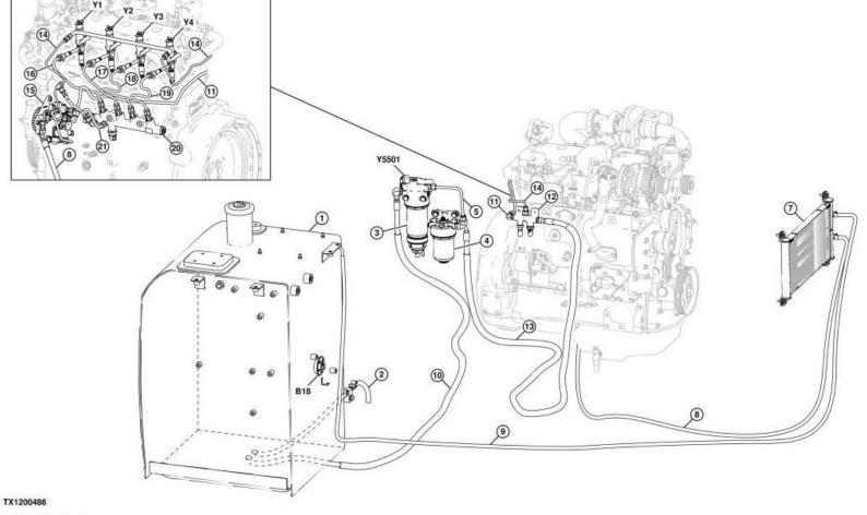
Engine Fuel System Component Location
