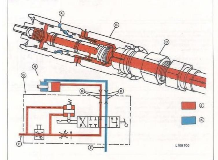
A-Leak-off passage B-Left-hand coupler C-Remote cylinder hose D-Right-hand coupler E-To sump F-From pressure control valve G-SCV housing H-Remote cylinder J-High pressure oil K-Return oil
