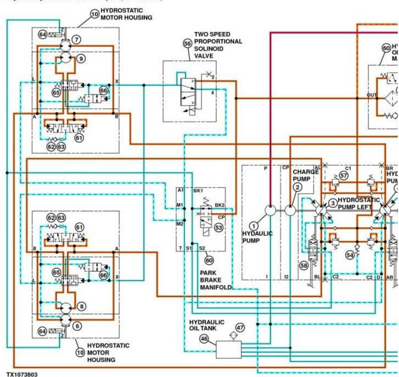
Hydraulic System Schematic-Two Speed (S.N. -150522)
