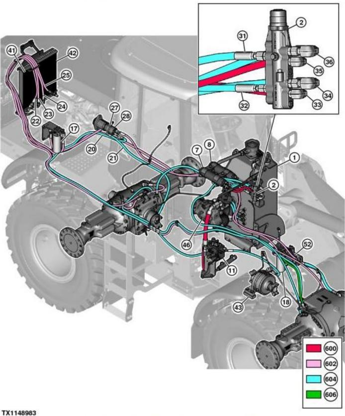
Service Brake, Park Brake, Differential Lock, and Axle Cooling Circuit Component Location
