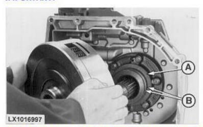
Before installing clutch to housing, make sure that seals (B) on transmission oil pump are properly installed and in good condition. Make sure thrust washer (A) is in place.
