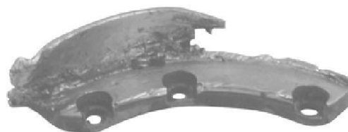
TX1080274A-UN: Chain Shot Guard—Edges Worn Away
