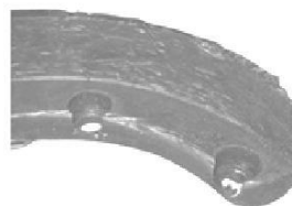
TX1080273A-UN: Chain Shot Guard—Worn Thin
