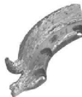
TX1080272A-UN: Chain Shot Guard—Peeled and Torn
