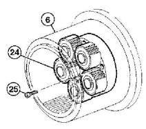
TX1028692-UN: Third Planetary Carrier Assembly
