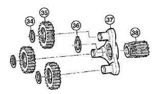
7. TX1029063-UN: Second Planetary Carrier
