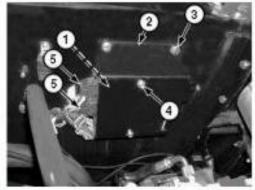
Engine Control Unit (ECU) Remove and Install
