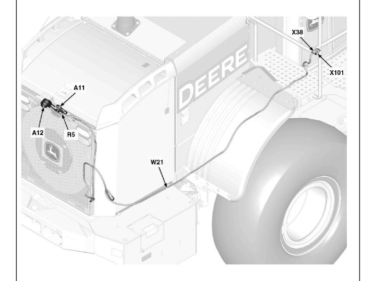
TX1146430A-UN: Radar Object Detection Harness (W21) Component Location LEGEND:
