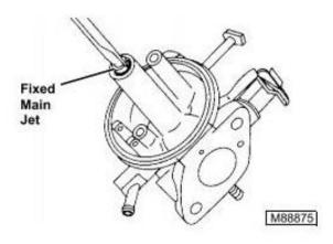
15. Install high speed nozzle and fixed main jet.
