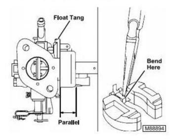
Hold carburetor in vertical position, with float hinge up. The float should be parallel with carburetor bowl mounting surface. If not, bend tang. DO NOT press on float to adjust.
