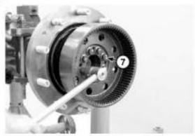
Internal Gear Cap Screws
