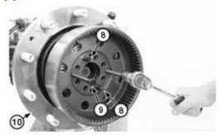
Internal Gear and Jack Screws
