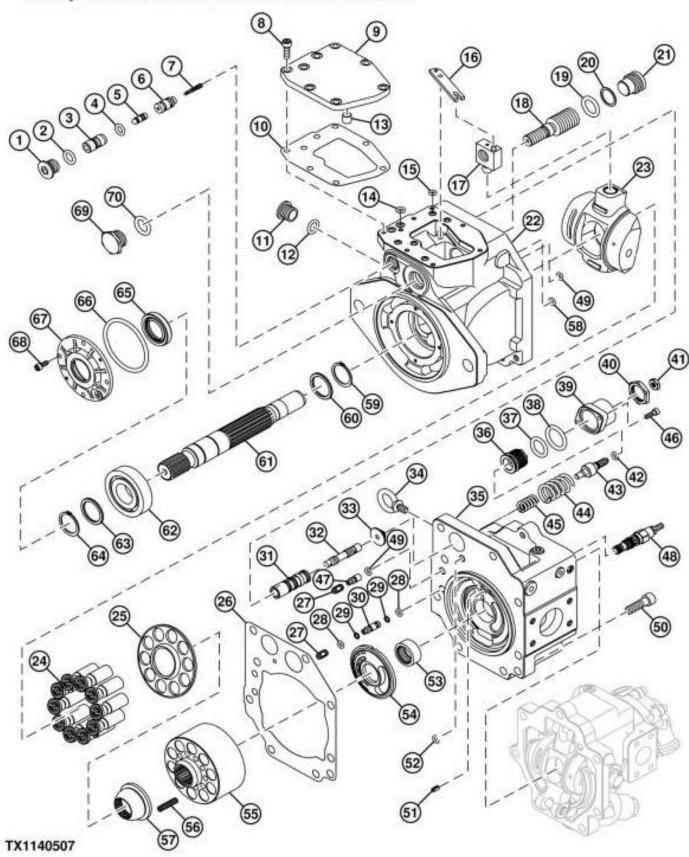
Pump 1 and 2 Disassemble
