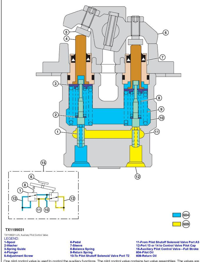
One pilot control valve is used to control the auxiliary functions. The pilot control valve contains two valve assemblies. The valves are controlled by movement of the pedals against the plunger (4). The ports (10, 11, and 12) in housing are identified by numbers and letters next to each port.
