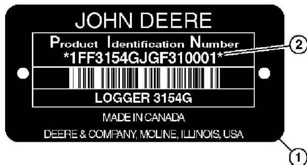
TX1217080-UN: Example of PIN Plate
