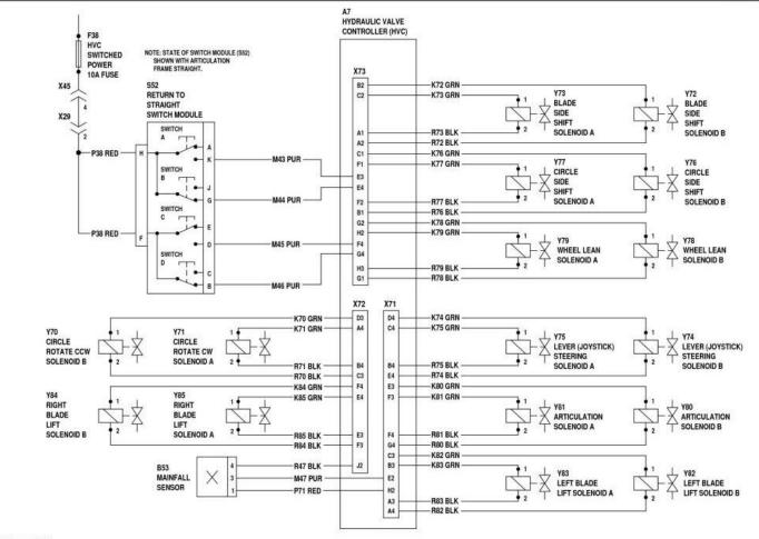
ydraulic Valve Controller (HVC) Circuit Schematic (2 of 2)
