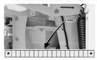
Serial Number Plate, 69X Series Rotary Harvesting Unit
