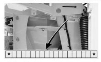
Serial Number Plate, 69X Series Rotary Harvesting Unit The serial number plate is located at the right side of the attaching frame.
