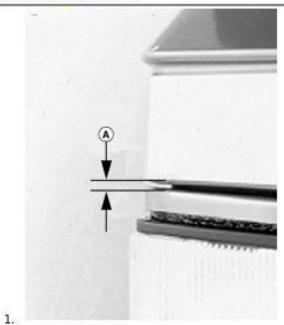
Check hood clearance (A). If clearance is more than 10 mm (0.394 in.), adjust hood latch height.
