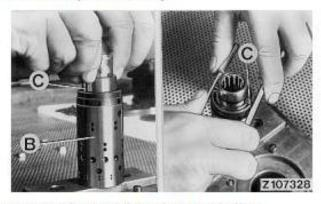
Insert Spring Pack into Sleeve and Align
