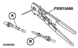
ZX008383-UN: Put Proper Size Contact on Wire and Crimp
