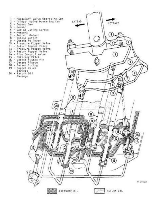
Fig. 3-Selective Control Valve Operation-Fast Extend
