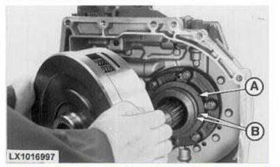
Before installing clutch to housing, make sure that seals (B) on transmission oil pump are properly installed and in good condition. Make sure thrust washer (A) is in place.
