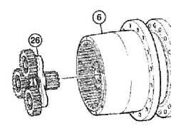
7. TX1028690-UN: Second Planetary Carrier Assembly
