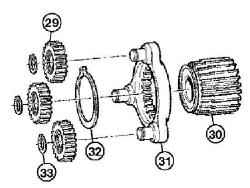
6. TX1029064-UN: First Planetary Carrier
