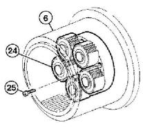
TX1028692-UN: Third Planetary Carrier Assembly
