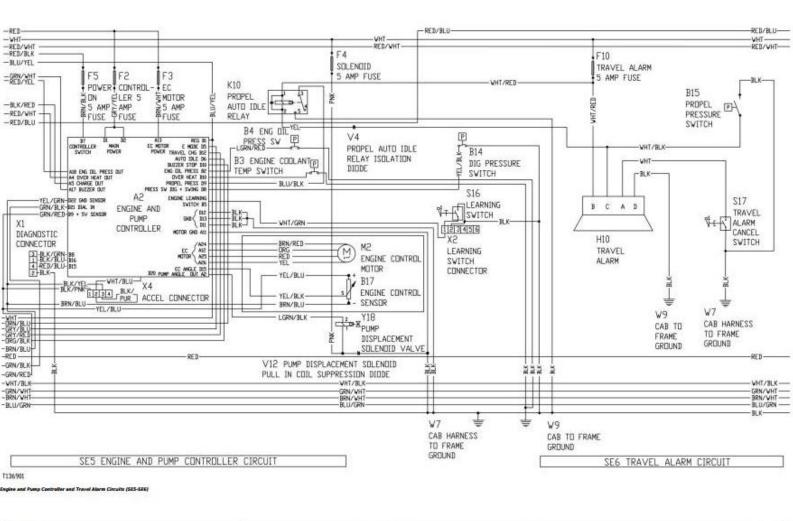
System Functional Schematic (SE5-SE6)
