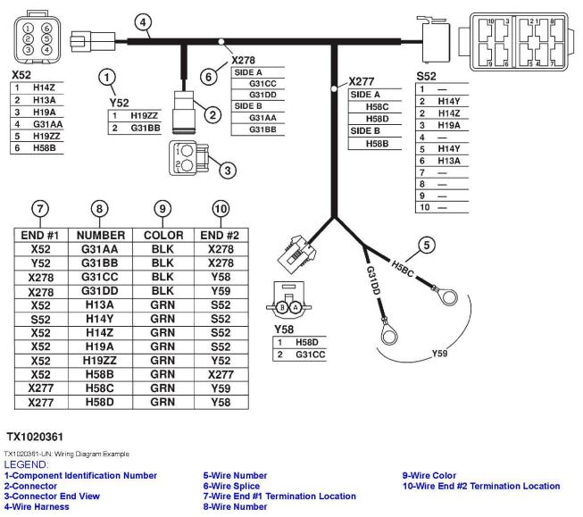
Each harness on the machine is drawn showing connectors, wires, and splices. A'W' component identification number identifies harnesses. (W6, Etc.) The harness is drawn showing spatial arrangement of components and branches.
