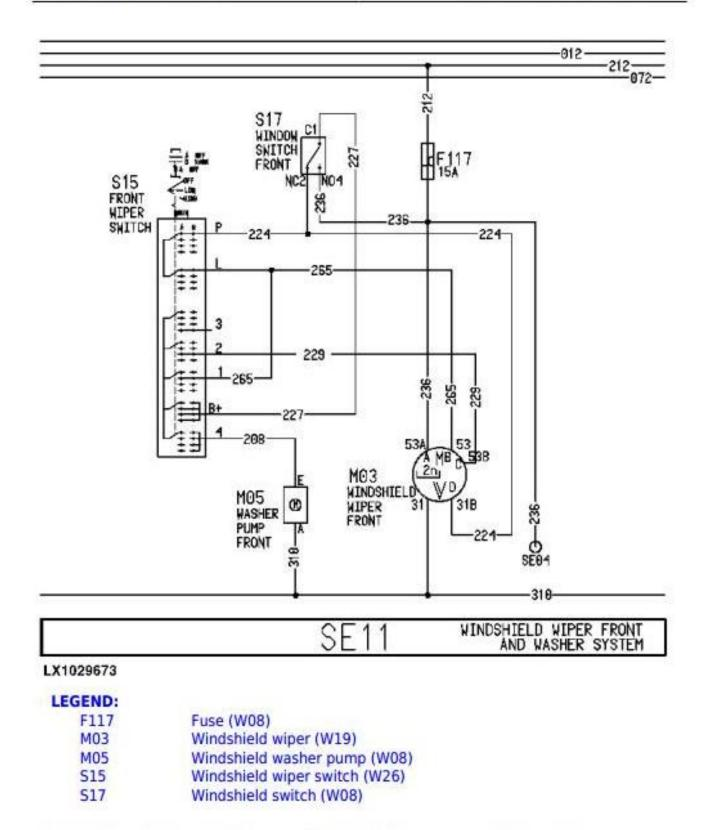
SE11-Diagnostic Schematic - Windshield Wiper and Washer
