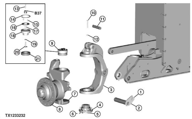
TX1233232-UN: Wheel Hub, Spindle, and Yoke—Non Six-Wheel Drive (6WD [right side shown])
