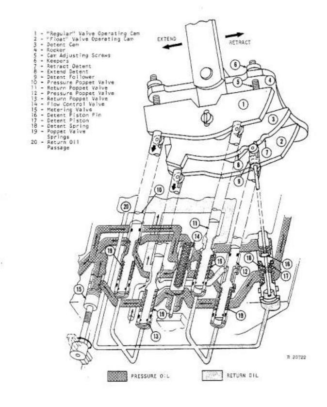
Fig. 3-Selective Control Valve Operation-Fast Extend
