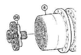
6. TX1028690-UN: Second Planetary Carrier Assembly LEGEND:
