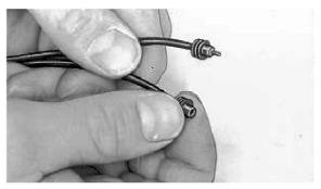
TS0136-UN: Install METRI PACK Male or Female Terminal Install METRI PACK Male or Female Terminal
