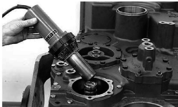
10. T160828B-UN: Bearing Bore Heat the bearing bore.
