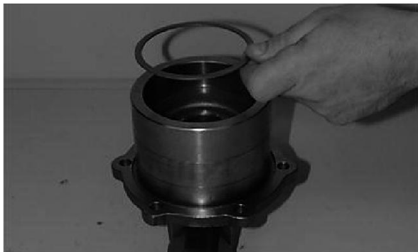
5. T160825B-UN: Shim Install shim.
