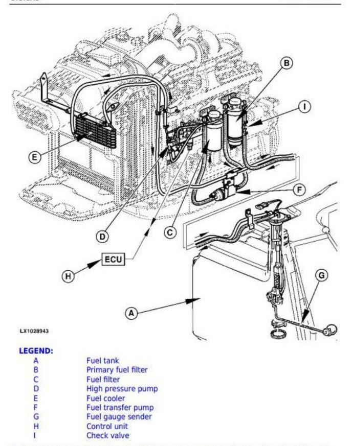
The fuel system consists of fuel tank (A), fuel gauge sending unit (G), primary fuel filter (B), fuel filter (C), high pressure pump (D), fuel cooler (E), fuel transfer pump (F) and control unit (H).
