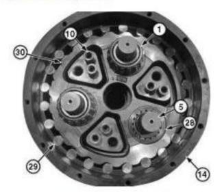
Travel Gearbox (one outer taper roller bearing removed for clarity)
