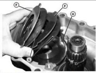
Remove the friction plates (F), friction disks (G), and brake actuator (H) from the rear axle housing.
