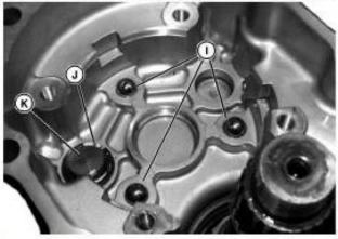
Remove three steel balls (I) from the rear axle housing.
